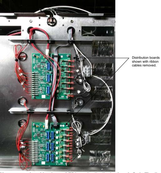
Upon startup, the cabinet beeps. LED's on the distribution boards flash. The displays show the version number of the cabinet's firmware and then the row's status.
