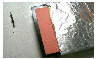
**Fig. 13:** The heater plate slides from the insulation.
