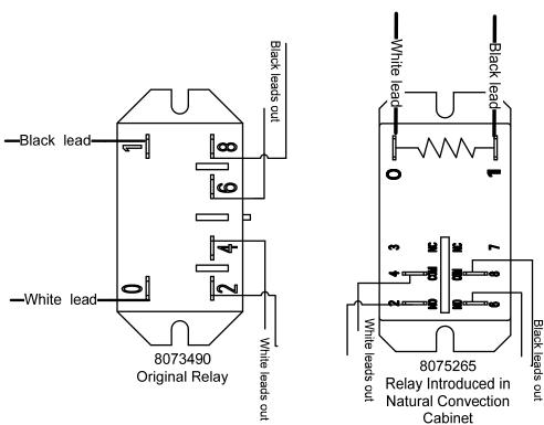
The natural convection (cabinet without fans) UHC-HD uses a different latching relay in the US. The new relay shares the same footprint as the original relay, but the terminals are laid out differently. (See diagrams above.)
