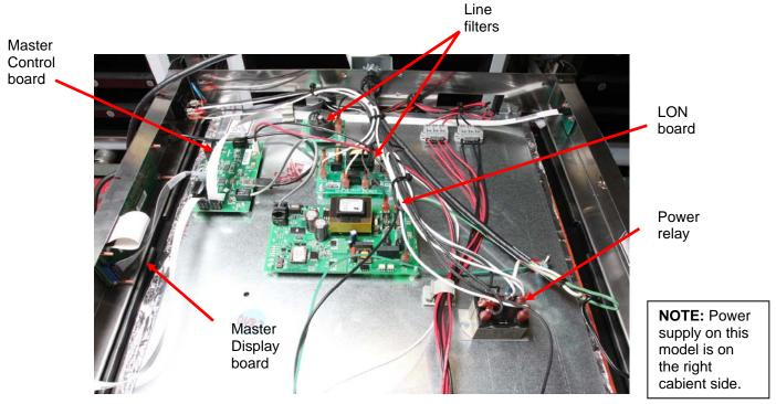
Figure 3: Natural convection design component shelf.
