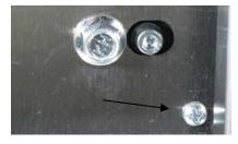
**Fig. 9** Loosen the hex bolt and remove the allen screw (arrows, upper photo). Some row positions may have an additional screw securing the bezel to the cabinet (lower photo). Push through the access port (arrow, upper photo), if necessary, to remove the bezel from the cabinet.
