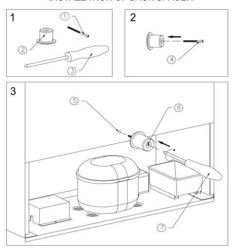
IMPORTANT - THIS SPACER MUST BE ATTACHED TO THE UNIT BEFORE INSTALLATION FOR VENTILATION PURPOSE. FAILURE TO DO SO VOIDS THE WARRANTY
