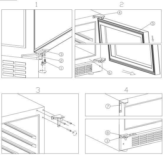
1 Lock screws 2 Lower hinge (Right) 3 Door axis 4 Top hinge (Right) 5 Door 6 Cabinet body 7 Top hinge (Left) 8 Lower hinge (Left)
