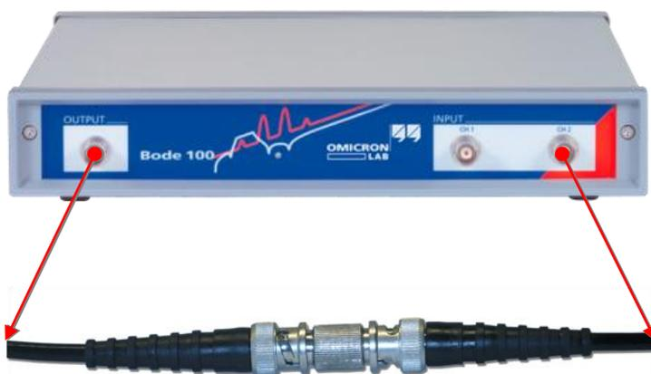
After connecting the cable the thru calibration can be done by clicking on User Calibration or Probe Calibration
