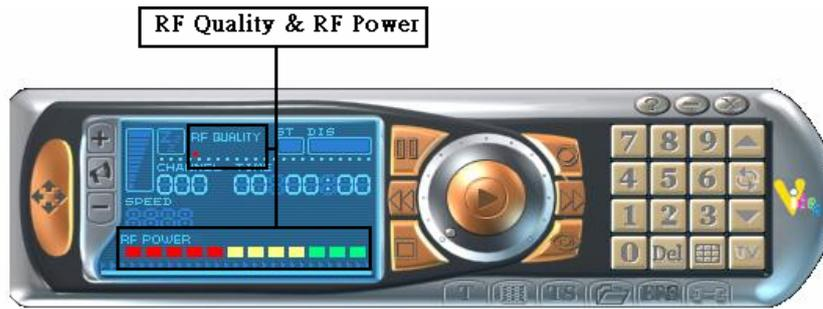
Please refer to the RF Power & the RF Quality indicating bars at the left side of the control panel on the screen, poor RF quality might result in no picture at all.
