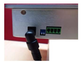
**Step 2.** Connecting the logger and (AP) Router with internet cable line.
