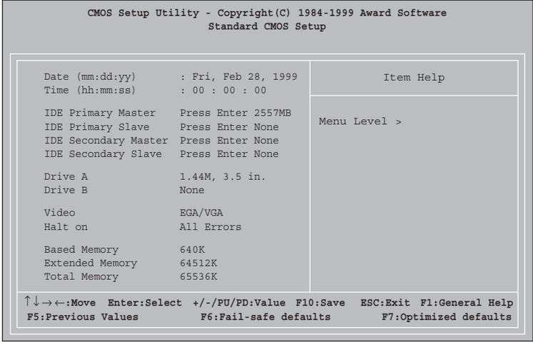
Figure 2-2: Standard CMOS Setup Menu
