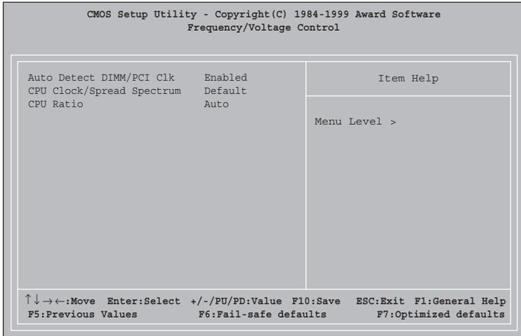
Figure 2-9: Frequency/Voltage Control Menu
