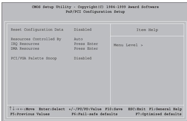
Figure 2-7: PnP/PCI Configuration Setup Menu
