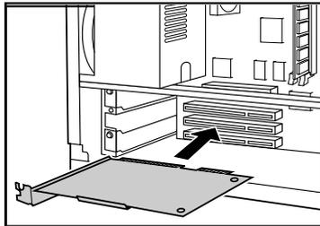
4. Secure the card to the housing with a screw.
