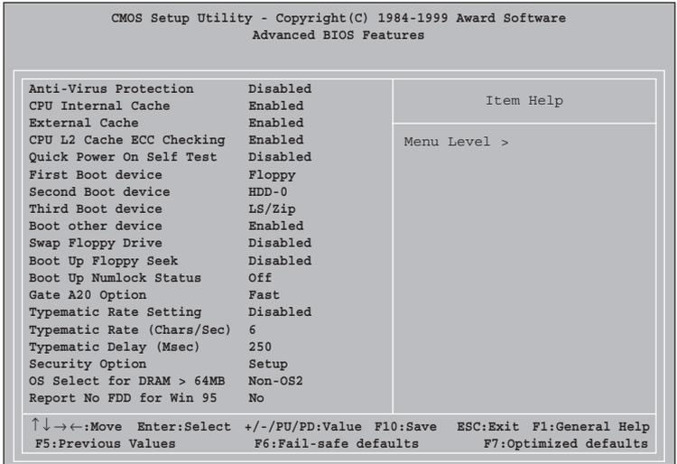
Figure 2-3: Advance BIOS Features Setup
