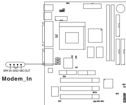
SPK\_IN is connected to the Modem Speaker Out connector.
