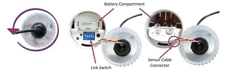
**Note:** When separating the base, be careful to ensure the sensor cable connector stays connected.
