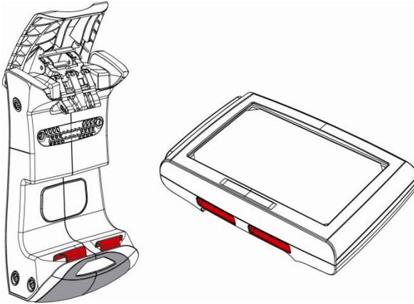
**1)** Present the Hawk II to the cradle. Seat the 2 rectangular slots in the side of the Hawk II (Adjacent to the TouchStar label) onto the corresponding seating keys on the Cradle. See picture for further info.
