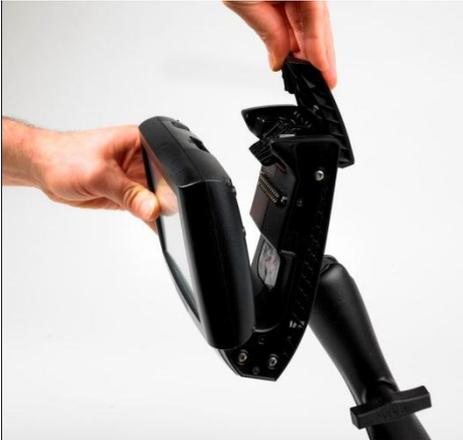
**1)** When removing the Hawk II from the cradle, lift the handle until it locks in the open position. The Hawk II is still held in position by the cradle, so the user can easily remove the unit.
