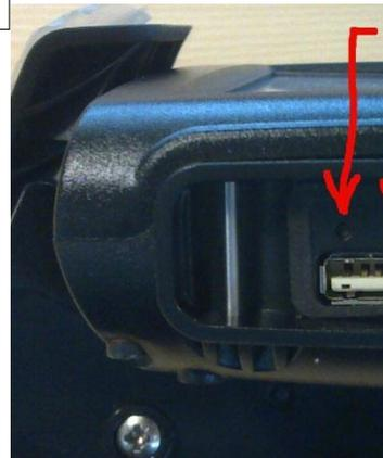
**Figure 2:** Position of reset and debug push-buttons, and debug serial port
