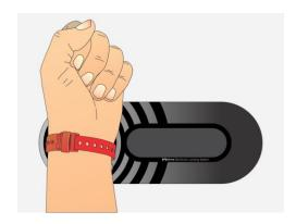
**STEP 1:** Approach the RFID media to the antenna field. Reading distance is 2-5 centimetres from the device surface. Hold the RFID media in the field for a few moments for device to read and process it.
