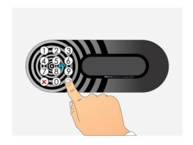
**STEP 1:** To enter Master mode press and hold the ✓ key for more than 3 seconds.
