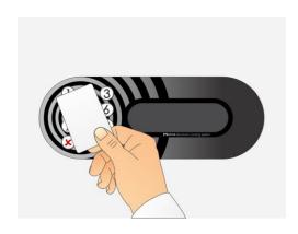
**STEP 1:** Approach the Master card to the antenna field. Reading distance is 3-5 centimetres from the device surface. Hold the Master card in the field for a few moments.
