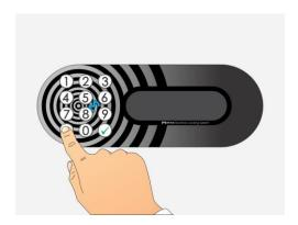
**STEP 1:** To enter Basic Setup mode press and hold the **x** key for more than 3 seconds.
