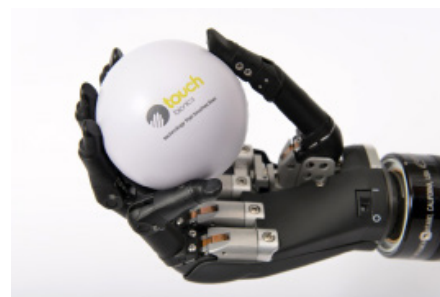
Figure 2. Compliant grip allows hand to take shape of the object
