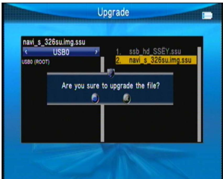
Warning: During the upgrade process, do not power off or pull out the USB Stick otherwise damage to the machine software will take place, can't re-boot.
