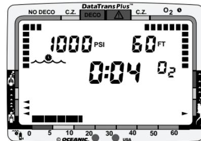
Fig. 104 - High Oxygen Accumulation (warning)
