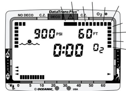
Fig. 105 - High Oxygen Accumulation (alarm)
