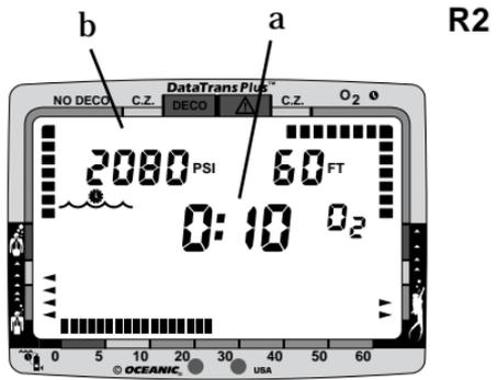
Fig. 15 - Oxygen Accumulation Time Remaining
