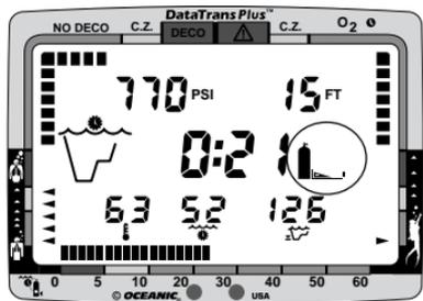
Fig. 107 - Low Battery (Transmitter)
