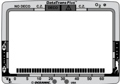
Fig. 11 - Breathing Gas Time Remaining Bar Graph
