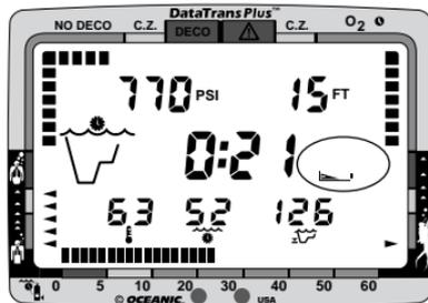
Fig. 108 - Low Battery (Display Module)
