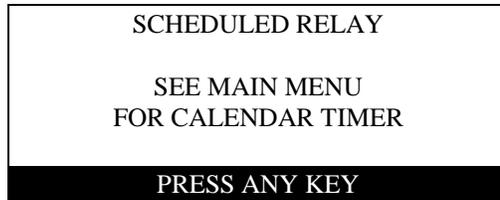
The relay has been configured to operate based on a Calendar Timer but, the relay will not activate because the Calendar Timer has not been programmed yet.
