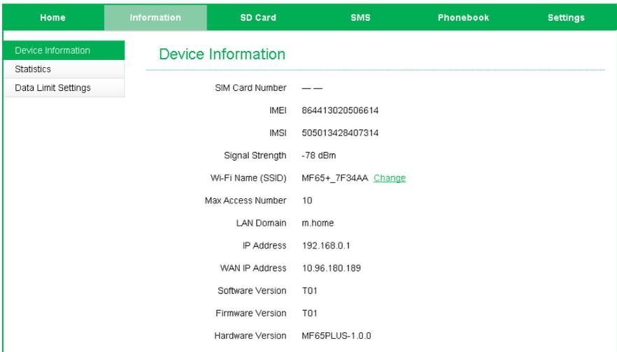
The Information tab shows the summary device status, how many devices are connected by Wi-Fi and whether you are connected to the mobile broadband network.
