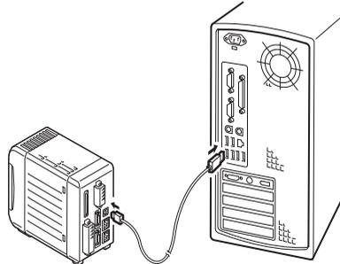
**1** Connect the Type-B connector of the USB cable to the controller.
