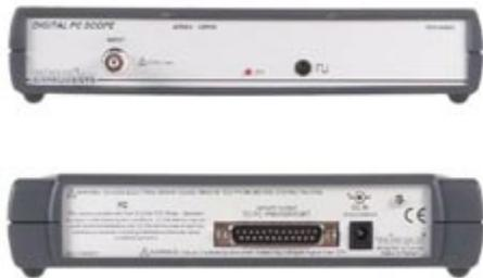
The PCS100 is a digital storage oscilloscope, using a computer and its monitor to display waveforms. All standard oscilloscope functions are available in the Windows program supplied. Its operation is just like a normal oscilloscope. Connection is through the computer's parallel port, the scope is completely optically isolated from the computer port.
