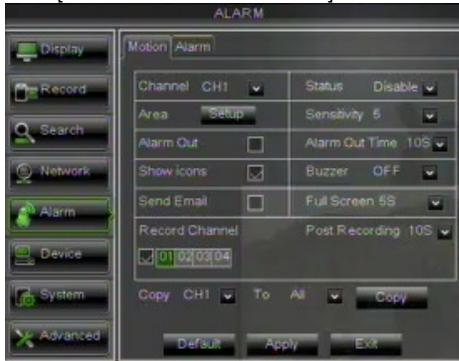
**Channel:** allow you enable/disable the motion function for any channel.
