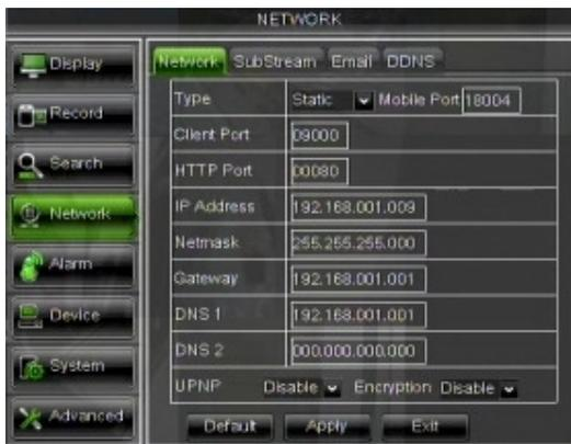
When selecting **Static** from the Type, user can directly input IP address, Subnet Mask, Gateway and DNS shown as above.
