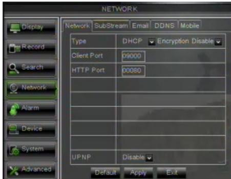
When selecting **DHCP** from the Type, A router will automatically allocate IP address for your DVR. After restarting each time, the IP address captured by your DVR may be different. So, port forwarding is required when you visit a remote DVR.
