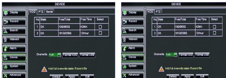
When DVR is connected to a HDD, the system will automatically detect if HDD is normal or not; If the cable connected to HDD is loosen or HDD is abnormal, HDD status will be shown as “No Disk”, or, If HDD need to be formatted, status will be shown as “no format”, otherwise, the HDD status will be shown as “Normal”
