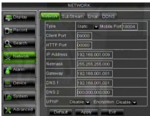
After selecting network mode - such as DHCP, PPPOE or static allocation- and setting up ports, you can visit DVR remotely through a network or internet.
