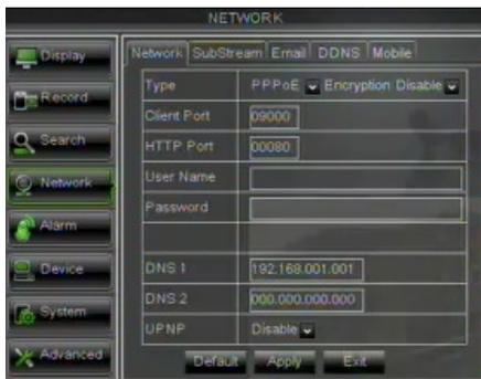
When selecting PPPoE form the Type, user can input user name and password provided by ISP and set Media and Web port. And now you can visit your remote DVR by using the IP address captured after registering a domain name and web port and connect to your DVR via public network.
