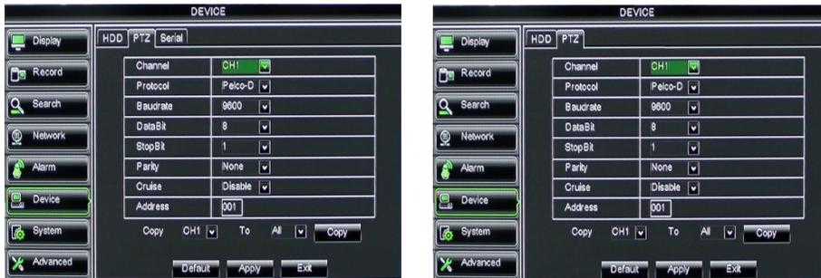
You could select the channel you desire to control and set PTZ protocol (Pelco-D or Pelco-P), Baud Rate (1200, 2400, 4800, 9600), Data bit (8, 7, 6, 5), Stop bit (1, 2), Parity Check (None, Odd, Even, Mark, Space), Address Code and Cruise status respectively. Please note the PTZ device can be activated only when a channel in connection with the PTZ camera is selected.
