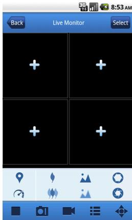
You need to Maximize a camera window and open PTZ mode to control the camera. Tap Arrows on the side of camera window to control camera move side to side or up and down. And other control buttons allow you to do Zoom, Force, Iris, PTZ speed and Preset, etc. As shown in the follow figures.
