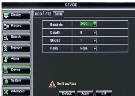
When operate DVR via keyboard, it is required to set communication protocol.
