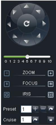
PTZ moving Direction control: allow you control PTZ camera's direction. And the middle button is called [Auto-cruise] button.
