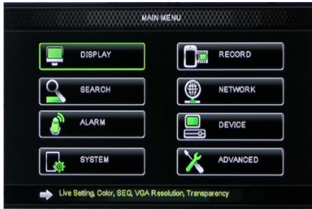
On <Live> mode, click [Menu] button on the front panel or Remote controller to enter into Main menu interface shown as above. And also you can click [Home] icon to enter the main menu screen. In Main Menu mode, you can control device management settings, such as Display, Record, Network, Search, Device, System and Advanced setting etc.
