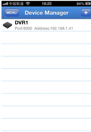
To add a new device, click "Add" button at the top right, then you can input the device name, address(IP or domain name), port, user name and password etc. The Channels property can be retrieved form device.
