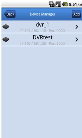
To add a new device, click "Add" button at the top right, then you can input the device name, address(IP or domain name), port, user name and password etc. The Channels property can be retrieved form device.
