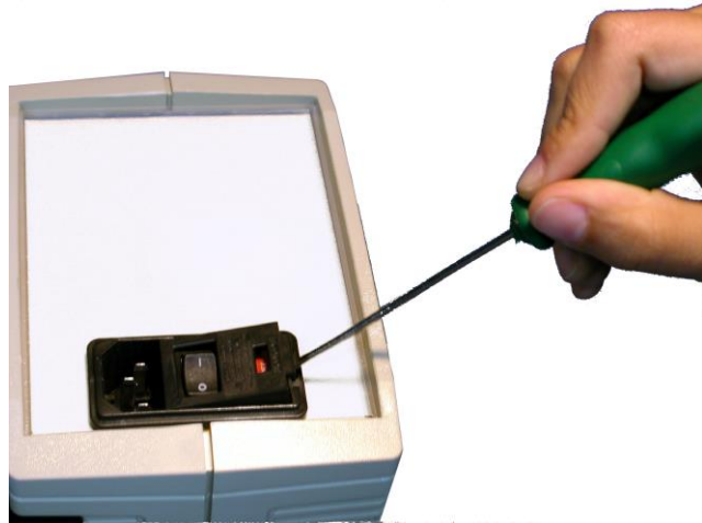
Figure 2. Open fuse-holder door.
