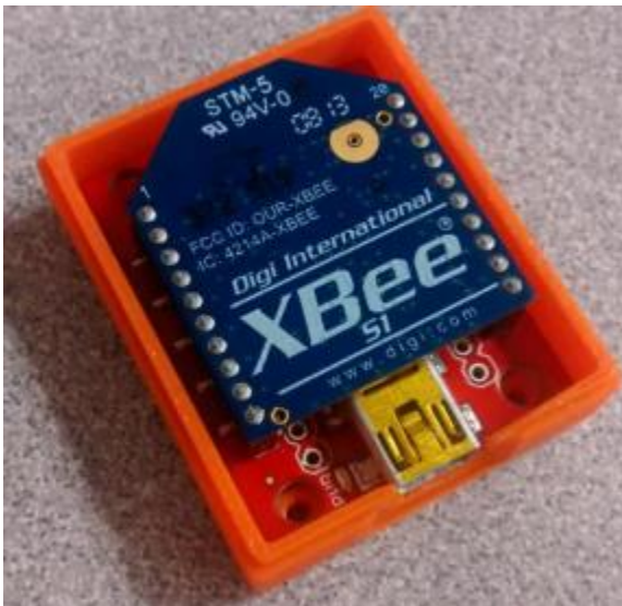
Figure 15: Xbee USB Explorer with Xbee module and 3D printed enclosure.
