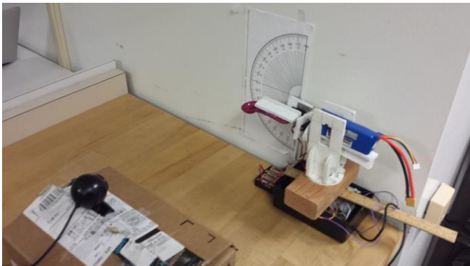
Figure 33: Test rig to observe linearity of A3020 servos.
