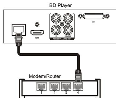
Using a wired network provides the best performance, because the attached devices connect directly to the network and are not subject to radio frequency interference.
