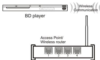
The network configuration and connection method may vary depending on the equipment in use and the network environment. This player is equipped with an IEEE 802.11n wireless module, which also supports the 802.11b/g standards. For the best wireless performance, we recommend using a IEEE 802.11n certified Wi-Fi network (access point or wireless router).
