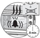
When cooking is completed, you will hear a beep and the timer automatically returns to the **Off** position, the power indicator light turns off.
