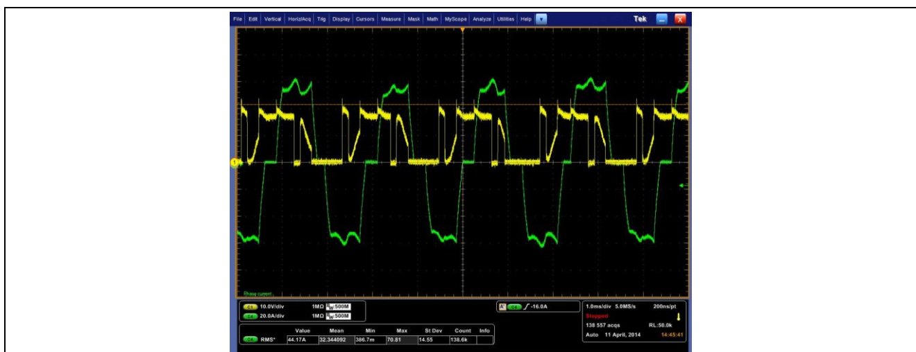
Figure 36 Phase voltage (yellow trace) and phase current (green trace) waveforms
