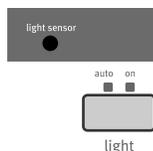
**Auto:** The light sensor monitors the light level in the room. The dispenser light will illuminate at half-power when the light level is low. To activate the Auto option press the “light” button. The Auto indicator light will illuminate.
