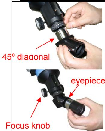
**Insert 45° diagonal:** Insert the diagonal into the eyepiece side of the telescope. Tighten the thumbscrews to a firm feel only.
