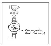
Connection to the gas supply should be made using the Aquaknect AS/NZS 1869 class B hose assembly with an internal diameter of not less than 10mm and regulator (regulator for use with natural gas)
