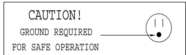
*This label is attached to the cabinet power cord on models with a power cord.*
