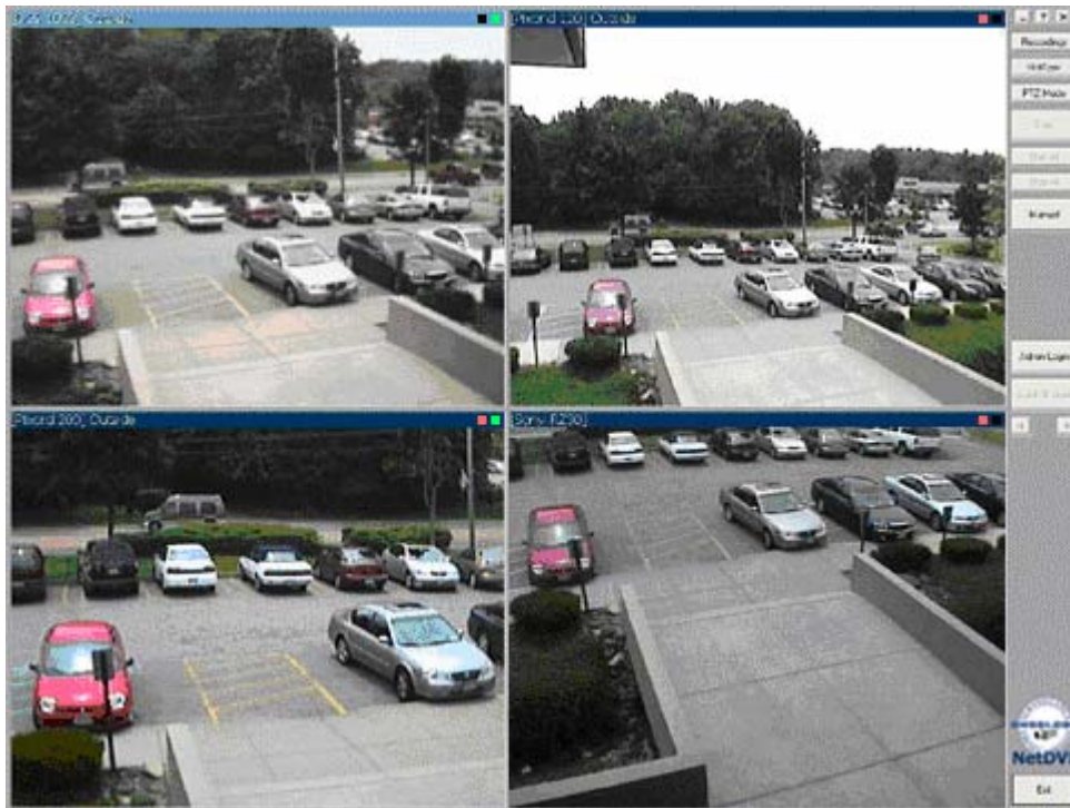
Figure 11: Main window of the NetDVR Monitor application. Here shown with four monitor windows, each showing the image stream of the associated camera) and the separate HotSpot feature enabled.
