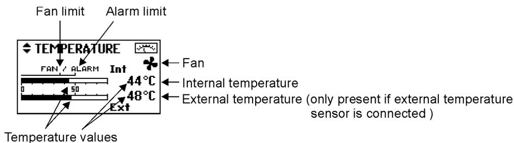
Figure 13-4: Temperature values and fan status
