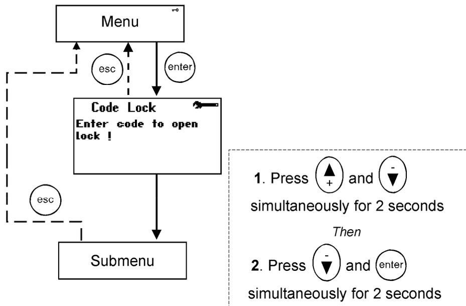
Figure 4: Entering a submenu with a keylock
