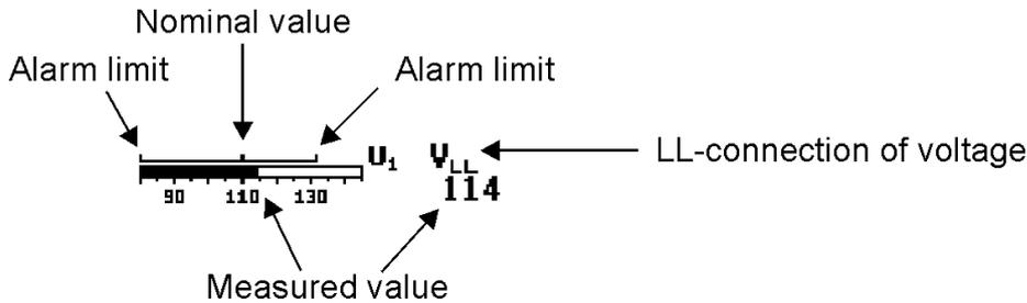
Figure 13-2: Measured value and alarm limits
