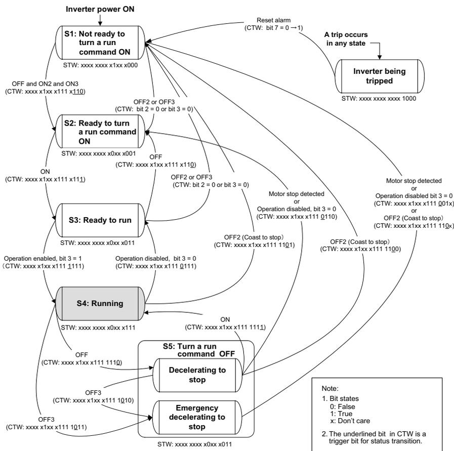
Figure 8.2 Status Transition Diagram of PROFIdrive Profile
