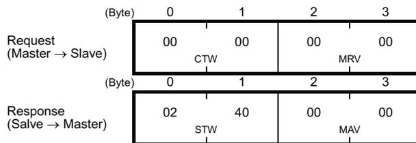
STW: Data 02 indicates that frequency and run commands from PROFIBUS are enabled. Data 40 indicates that the inverter is not ready to turn a run command ON.
