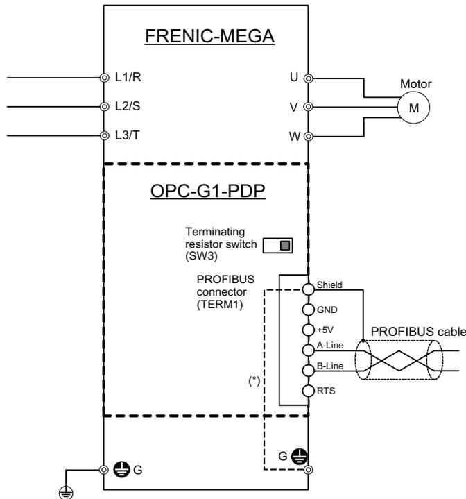
(\*) Mounting the communications card on the inverter forms this connection.
