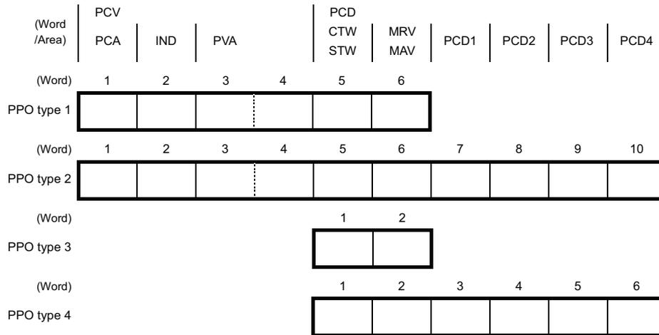
Figure 8.1 Data Formats of PPO Types Supported
