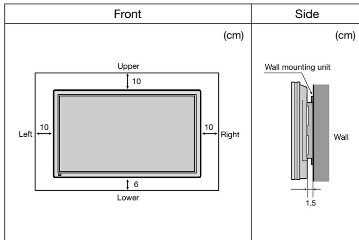
When using the wall-mounting unit (vertical type)
