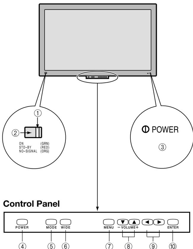
The control panel opens when you press the lower center of the display.
