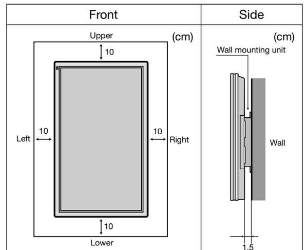
\* When you install the display lengthwise (rather than in its normal position), you need to adjust the display so that characters will appear properly.
