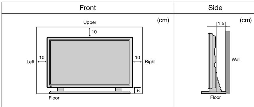
When using the wall-mounting unit (horizontal type)
