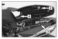
To mount the seat, place it on the motorcycle and position the hooks [2] on the bottom of the seat behind the dollies [3] on the subframe. Press down on the seat near the holding strap while sliding it forwards. The two tabs [4] must hook onto the tank. Turn the ignition key in the seat lock 90° in a counterclockwise direction and pull off. Check whether the seat is mounted correctly.
