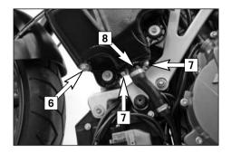
Remove the drain plug **[6]** on the oil tank and allow the oil to drain into a receptacle. Remove the screws **[7]** and tilt the oil return valve **[8]** to the side.
