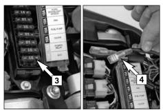
The ACC fuse [3] is designed for accessories with a maximum power consumption of 10 amperes. A connector [4] to connect the equipment is provided under the seat. Ask your authorized KTM workshop for details.
