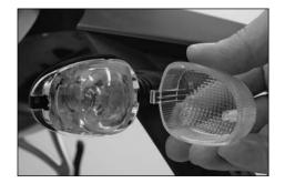
Slightly depress the bulb, turn it approx. 30° counterclockwise and pull it out of the socket.
