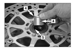
Before you remount the front wheel, clean and grease the shaft seal rings [5] and the bearing surface [A] of the distance bushings and mount the distance bushings (wide distance bushing in the left shaft seal ring). When mounting the distance bushing, be careful not to press the sealing lips towards the inside. position the front wheel according to the running direction shown by the arrows [B] on the rim.
