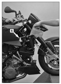
To completely bleed the cooling system, the motorcycle must be raised approx. 50 cm (20 in) in the front.
