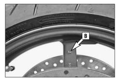
To remount the front wheel, lift the wheel on the fork and mount the wheel spindle. Mount the collar screw [2] and tighten slightly, tighten the clamping screws [3] on the right fork leg axle passage to prevent the wheel spindle from turning and tighten the collar screw to 60 Nm.
