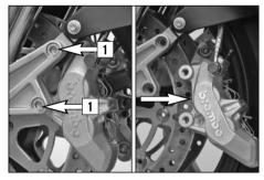
To remove the left and right brake caliper, remove the two screws [1] on each caliper and pull the brake caliper off the brake disk towards the back.
