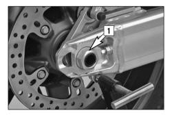
Unscrew the collar nut [1], remove the chain tensioner [2], hold the rear wheel while you pull out the wheel spindle [3]. Push the rear wheel forward as far as possible and remove the chain from the rear sprocket. Carefully take the rear wheel off the swing arm.
