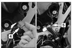
Mount the oil drain plug on the oil tank with a new seal ring and tighten to 20 Nm.
