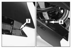
Fit the slots in the front spoiler on the lower screws [7] and tighten. Apply Loctite 243 to the side screws [8] and tighten to 10 Nm.
