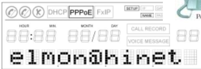
5.1.1.1 When asked to enter the account name (display will show **Account Name** for two seconds), press the numerical keypads to make up to 29 alpha-numeric characters while **SETUP** and **NAME** are on. Press <Clear> to erase the last entry, <Exit> to ignore entries and return to [Standby](#) mode, or <OK> to store the account name to the system table.
