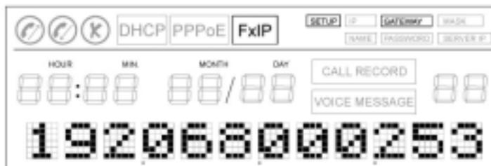
**5.1.2.1** When asked to enter the PeerCall IP address (display will show **PeerCall IP** for two seconds), press the numerical keypads to make the right entries while **SETUP** and **IP** are on. Press <Clear> to erase the last entry, <Exit> to ignore entries and return to **Standby** mode, or <OK> to save the entry.
