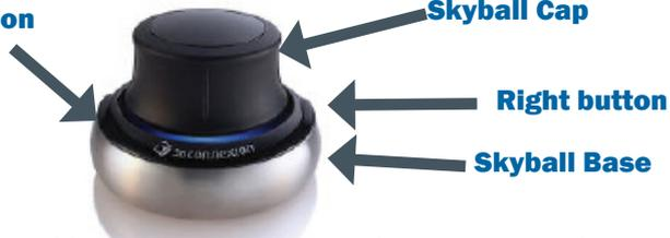
The Skyball enables you to pan, zoom, and rotate separately or at the same time. The base of the Skyball does not move, only the cap (top half), moves.
