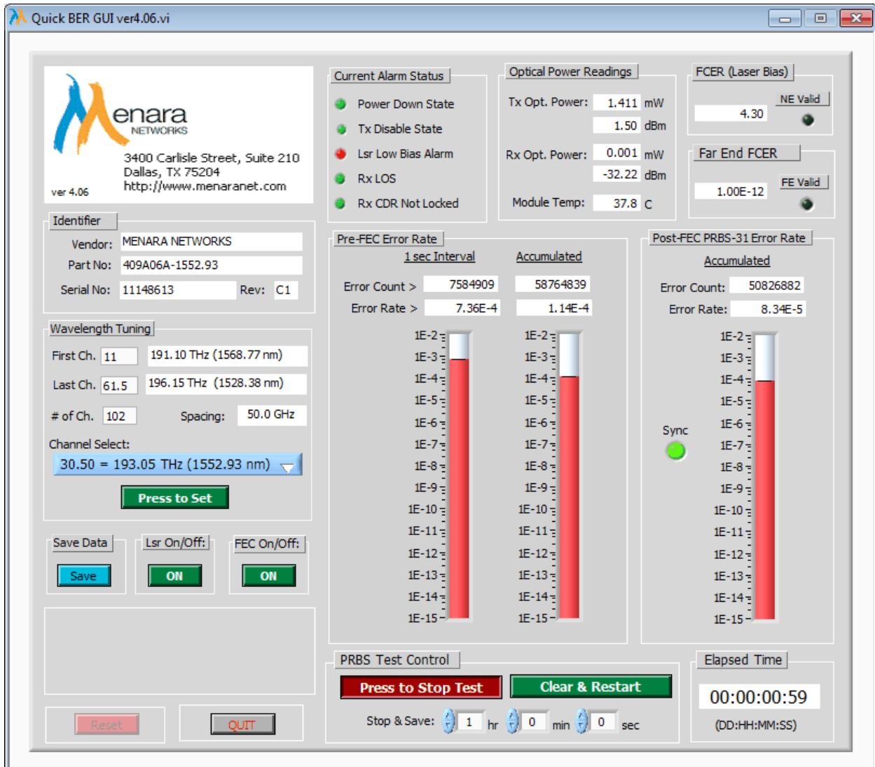
Figure 18: Pre-FEC and Post-FEC BER Test with High BER
