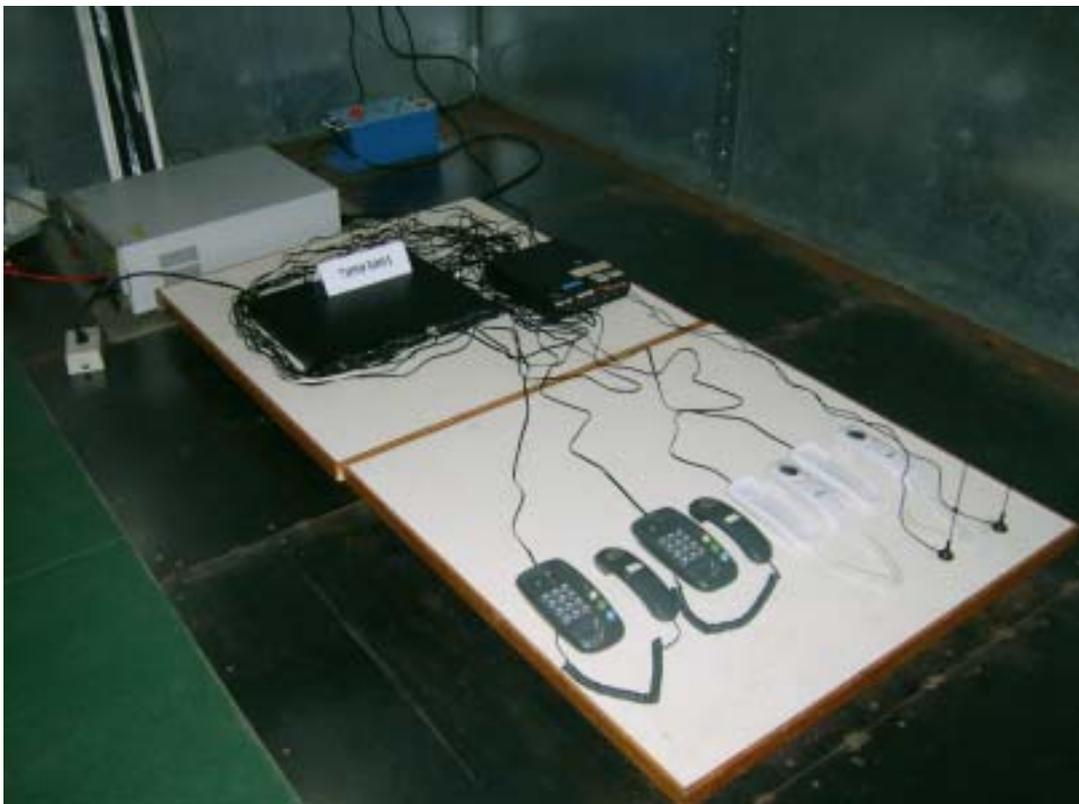
**EFT For I/O Test**
