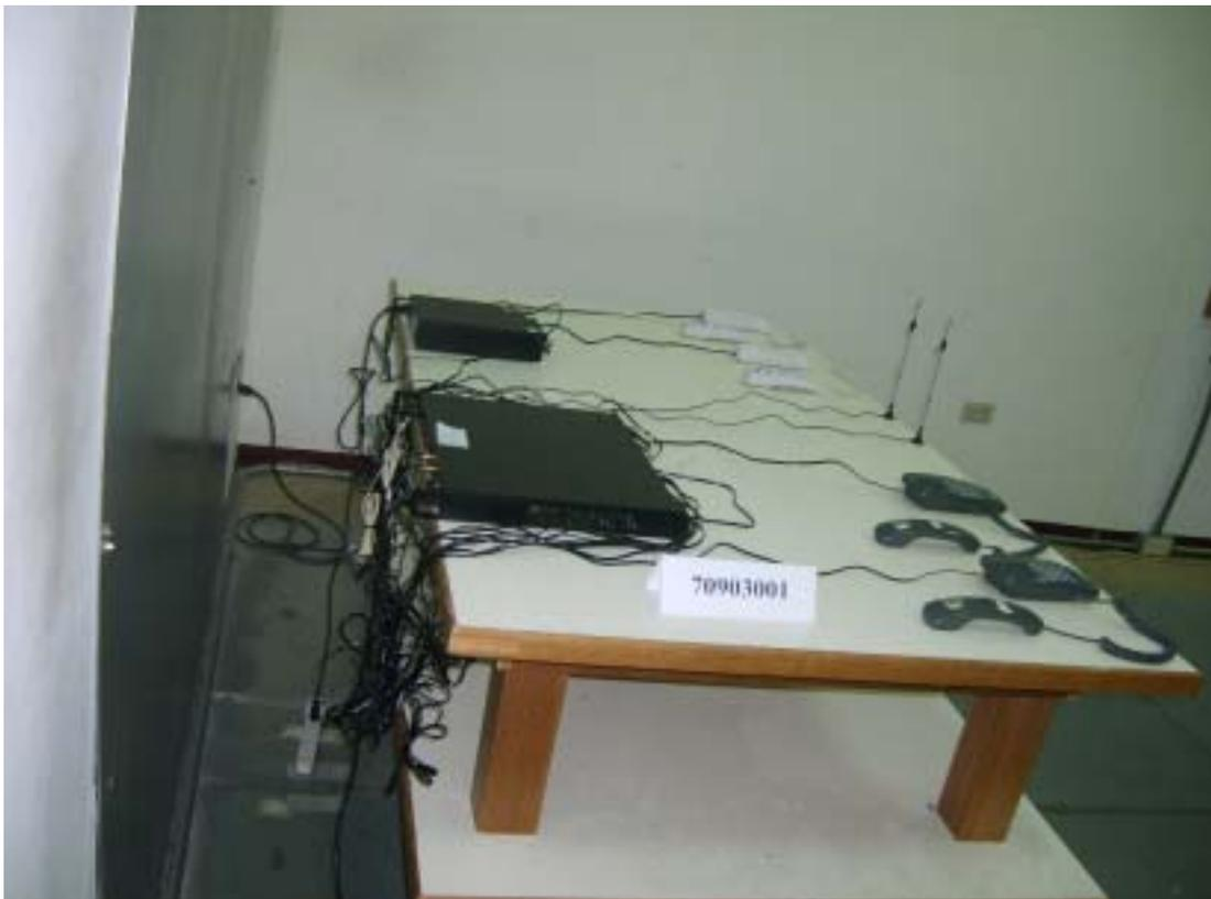
**CONDUCTED EMISSION TEST AT TELECOMMUNICATION PORTS**
