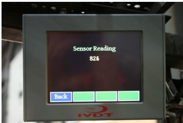
*If the above test is valid than the system and pressure transducer electrical connections are done right. The next procedure will be to calibrate the SkidFleet weighing function*
