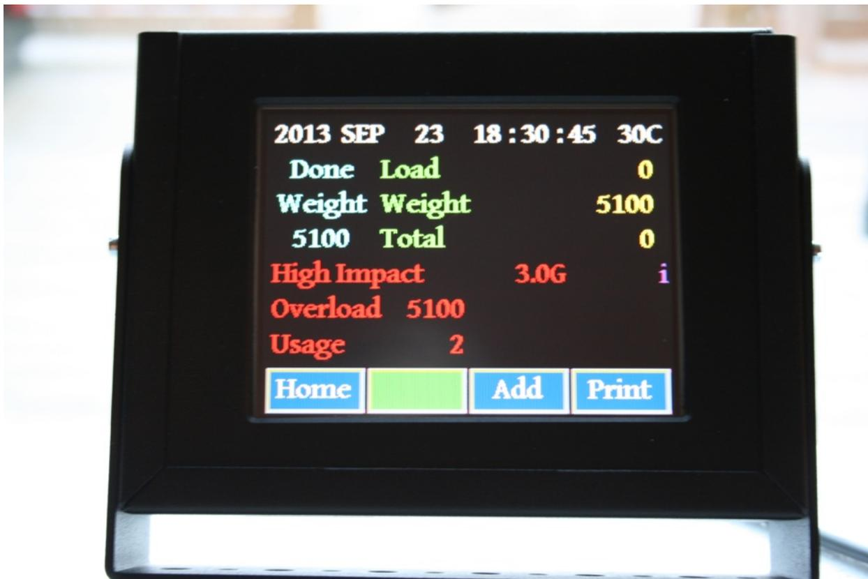
**i sign (purple color) shown on LCD display indicates that Impact module is active**
