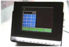
2. Enter number **999** and press **Enter key** to start the procedure of the input mode for a valid operator ID#'s.
