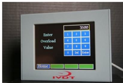
SkidFleet systems with overload warning function will have LCD screen advance automatically to “Enter Overload Value” after the calibration of loaded forks with known load weight is finished. At that point enter the overload warning value for your vehicle application and press Enter key.
