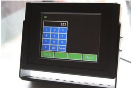
With a standard Operator ID# the end user can input into the system **any ID# from number 1 to 999**. System will register the operator ID# and you will be allowed to proceed to the next step.
