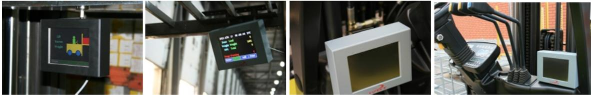
There are many examples of mounting locations that will depend on the vehicle model. However, additional mounting items such as a flat brackets may be needed to help secure the unit to upper right corner of the guard or side railing.
