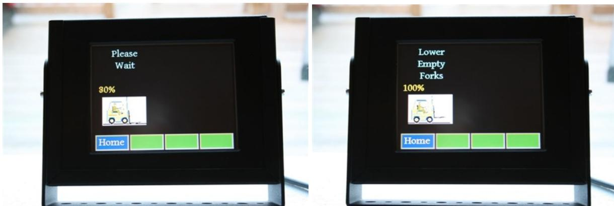
Activate lift control valve and “quickly” lift empty forks. Do not lift empty forks slowly !
