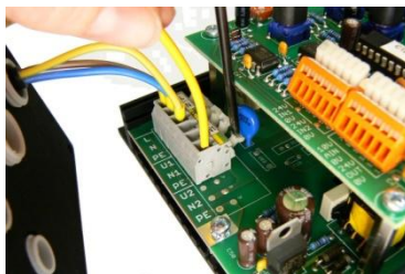
Fig. 8 - connecting conductors to terminals
