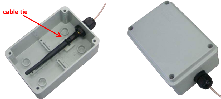
Figure 6-5 Outdoor installation; example of CDD radio antenna mounted inside a plastic box with watertight seal
