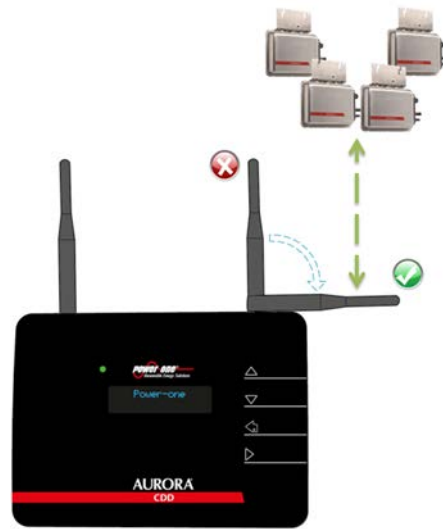
Figure 4-2 Correct orientation for CDD radio antenna, sideways to the AURORA MICRO inverters
