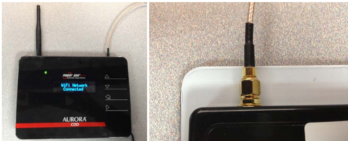
Figure 6-6 AURORA CDD with radio signal extension cable attached, top view (left) and bottom view closeup (right)
