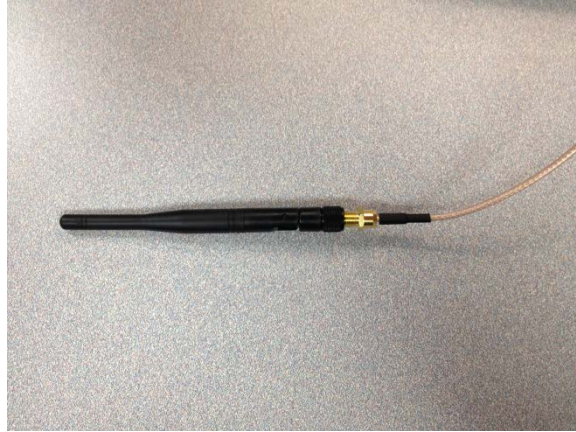
Figure 6-3 45' radio antenna extension cable attached to radio antenna
