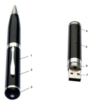
1- mic 2- lens 3- Shutter button 4- LED status indicator 5- reset
