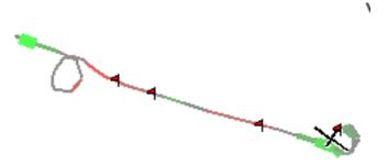
If Vega or an intelligent variometer is connected with Netto output, the Netto vario value is used; hence the colours and thickness of the trail indicates the air-mass vertical movement rather than the glider's vertical movement.
