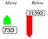
The scale of the final glide bar is  $\pm -500$  meters.
