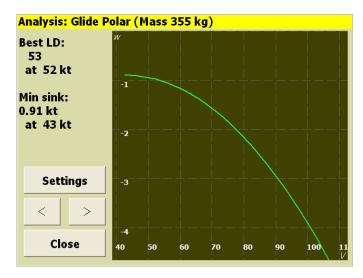
In this dialog page, the 'Settings' button opens the flight settings dialog (e.g. to adjust the bugs/ballast).
