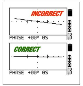
On irregular mineralization soils, for instance on a plow land, the device cannot always be accurately balanced in the automatic mode, because when a vertical balancing is performed, there is one soil under the searchcoil (a clod or an air layer) and during scanning these pieces go one after another, sometimes it leads to phantom responses of the device identification channel. At the same time, ground phase digit in automatic balancing operation may differ by 3 degrees on the same place.
