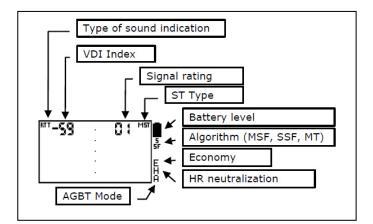
VDI means Visual Discrimination Indication. VDI Index This is a socalled electrical conductivity indication of the object. Angle between the vertical axis and main direction of the curl hodograph located in the left part of the screen has negative VDI and the right one has positive VDI Signal level - signal amplitude from the object in arbitrary units.
