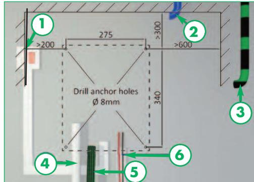
Minimum distances to the ceiling and to the sides are to be adhered to for the purpose of installation and maintenance. The control panel is fastened with four screws M 6 x 40 (wall anchors Ø 8 mm), ensure all 4 screws are used in order to avoid vibrations. Make sure that the correct types of wall plug are used for the wall material.
