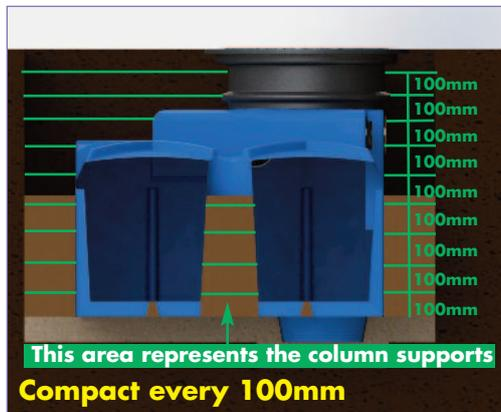
Ensure that the top of the tank is covered with at least 100mm of the filling material before filling the remaining (minimum) 400/800mm of the hole, bringing it up to ground level, with a material of choice suitable for the location of the tank.
