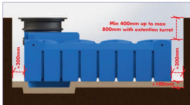
Carefully lower the tank into the excavation. Install and connect up all pipework, including the service duct for the floating suction hose and cabling.
