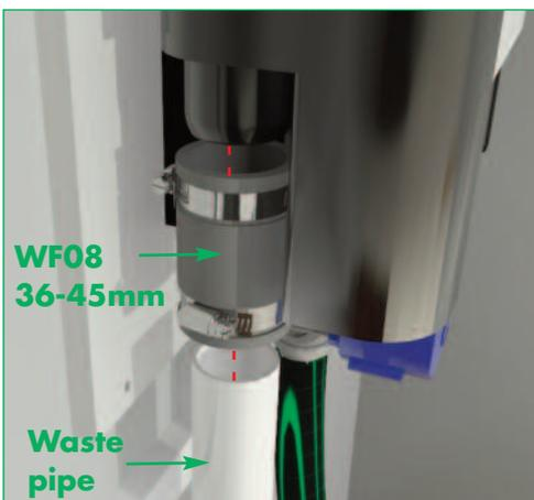
Using a WF08 36-45mm (not supplied) fitting connect a 43mm waste pipe (not supplied) to the overflow of the mainswater tank as shown. Run the waste pipe to a nearby drain, this will prevent water spilling onto the floor should the system overflow. The fitting and waste pipe are available from [www.floplast.co.uk](http://www.floplast.co.uk)
