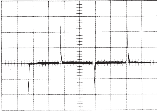
Figure 9 Correct Pole/Zero Compensation
