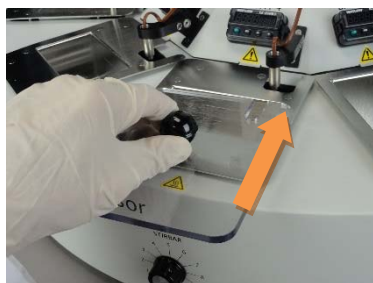
Insert a preheating bath cover to achieve high temperatures and reduce evaporation.
