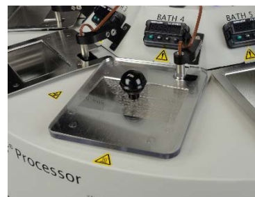
Insert a preheating bath cover to achieve high temperatures and reduce evaporation.
