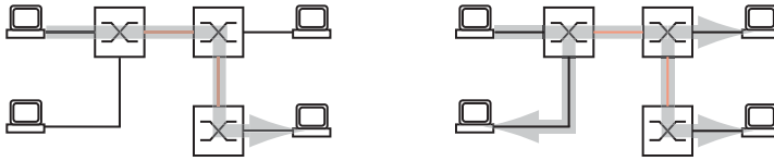
Figure 2: MAC Data Transmission: Unicast Data Packet (left) and Broadcast Data Packet (right)
