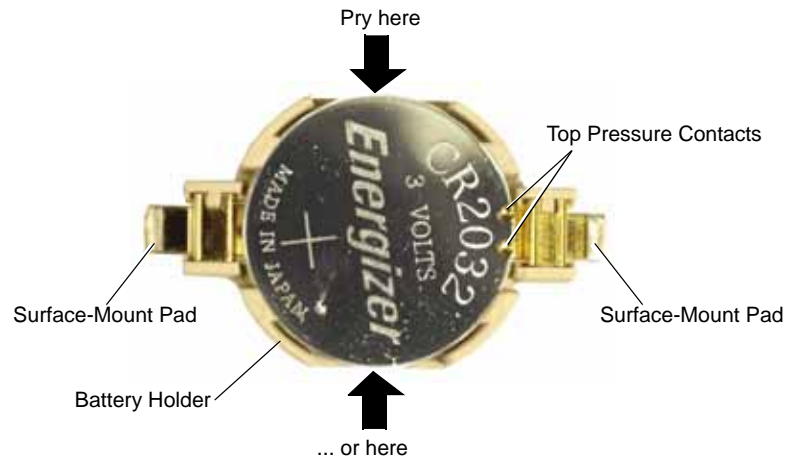
Figure 4-7. Removing the T2BC Lithium Battery
