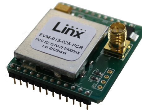
Figure 1: 25 Series Evaluation Module
