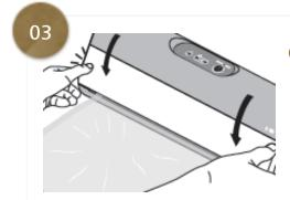
Open the cover and put the roll on the heating line, pushing the buttons on either side until clicking
