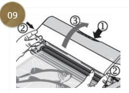
Pushing the (1)<u>vacuum removal button</u>, press the (2)<u>cover-release buttons</u> on both ends of above cover and open the cover to take out the poly bag.
