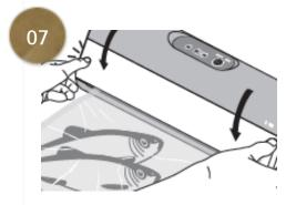
Put the other side which is not yet sealed in the below part of the chamber and close the cover and tap the both buttons on the both edges in turn until clicking.
