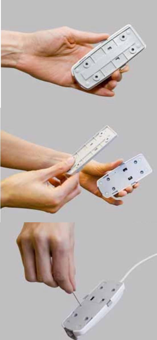
3. At the bottom of the ControlBox a small hole can be seen. To reset the default IP address insert an appropriate tool into the hole pushing it to the bottom.
