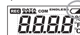
Battery Warning Mark
